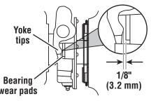
To change the yoke finger and bearing wear pads clearance, adjust the upper pedal stop to raise or lower the pedal in the cab.
