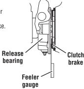
4 Slowly let up on the pedal and check the pedal position at the moment the gauge can be removed.
