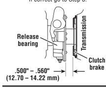
To change bearing position, you must internally adjust the clutch. Push pedal and hold pedal down when adjusting. Follow instructions for Kwik-Adjust or Value Clutches.
